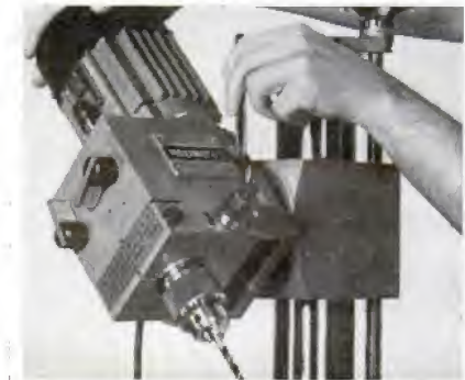
DRILLING-MILLING HEAD rotates 360^\circ in its mount. The rotating column permits compound-angle settings
